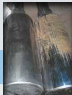
2 plungers that pumped tar with grit for 6 months (LEFT) New Carbide Coating (RIGHT) New Chrome
