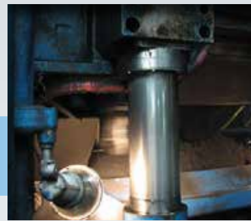
Carbide Coating after 5 years of use
